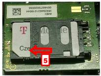
Note: All programmed parametres are saved on the SIM. The SIM you can insert into GDI already preprogrammed or setup GDI after switching ON (via bellow).
